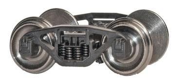
Many freight cars built in the 1920s were equipped with Dalmantrucks. The Dalman 2-level truck design used additional springs to give a smoother ride. Railroads using
